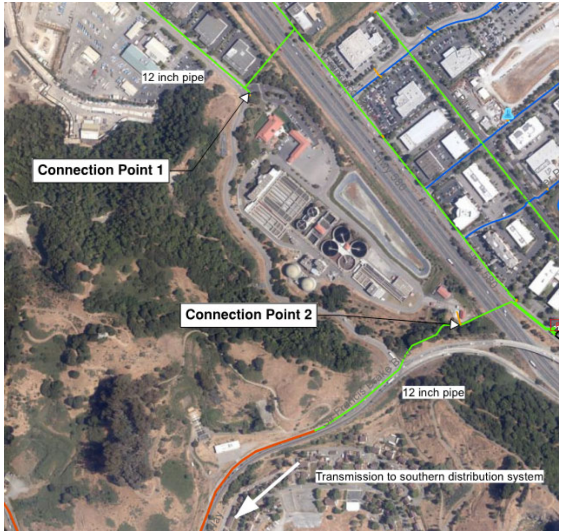
Figure 5.3 Proposed Connection Point Options to Existing MMWD Water Distribution System
